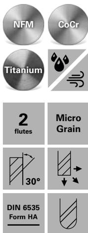
**End mill type:** Ball nose 180° bevelled pointed
